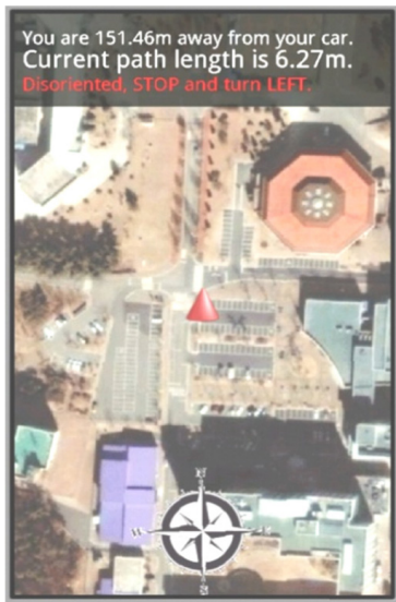
(Figure 8b) Whenever a disoriented step is detected, the user is informed and corrected.
