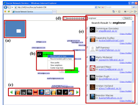
(Figure 6) Screenshot of the user-interface showing a mini map, a context menu, neighbors, a zoom-level bar and search results
