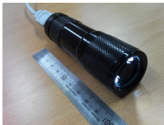
(Figure 6) Packaged camera module inside a cylindrical Aluminum case.
