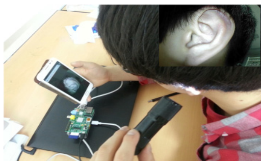
(Figure 13) Observation of an ear using WiFi-based wireless endoscope.
