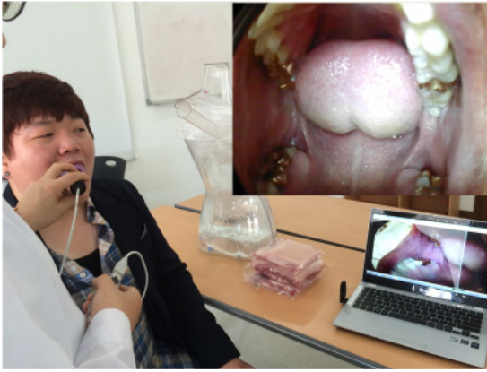
(Figure 10) Observation of an oral cavity using the UWB-based endoscope module.
