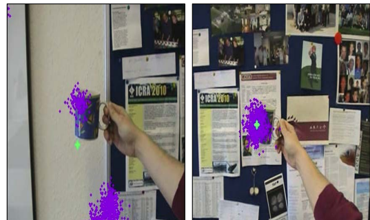
(b) Result of particle filter using HOG (Frame : 25, Frame: 100)
