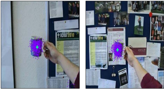
(c) Result of proposed particle filter using edge observation model (Frame : 25, Frame: 100)
