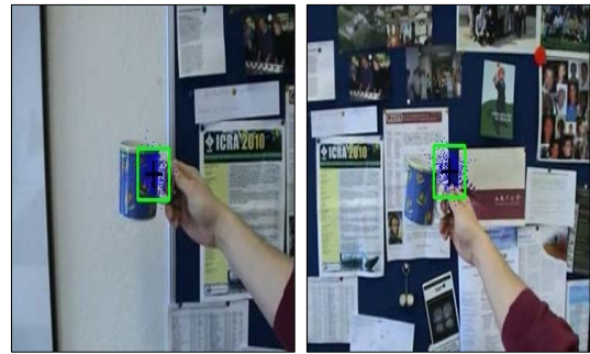
(a) Result of particle filter based on HSI color model (Frame : 25, Frame: 100)
